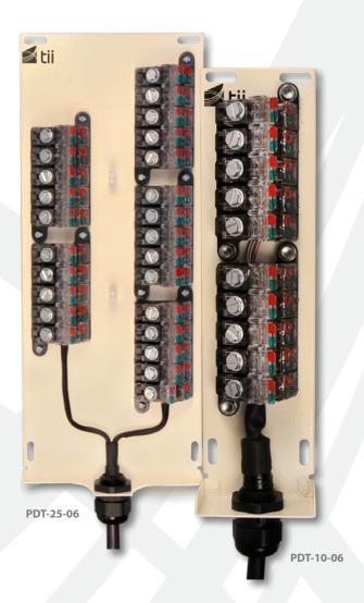
PDT Series are unprotected sealed terminals ideally suited for mounting within pedestals. Utilizing Tii's gel sealed tool-less IDC connections. The connectivity modules support drop wires from 18-24 AWG without the need to strip the insulation. The units are available from in both a 10 pair and 25 pair version.
