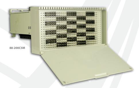
88-(XXX)C Equipment Terminal Blocks are used to terminate the exchange equipment pairs on the horizontal side of a conventional main distribution frame (MDF), and provide the cross-connect field for jumpering to the Outside Plant (OSP) vertical side of the frame. They also feature CAT5 compliance for superior transmission of DSL signals and other high frequency circuits.
