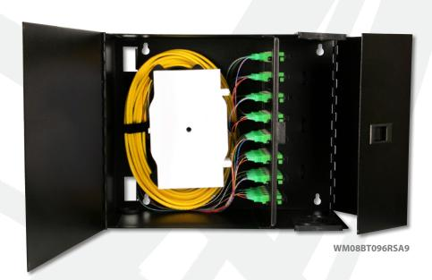
Wall mount fiber distribution unit designed to support patching and splicing in one unit. The enclosure has 8 adapter panel positions, allowing for a wide variety of fiber termination connector types. Two compartments separate the network terminations from the distribution terminations.
