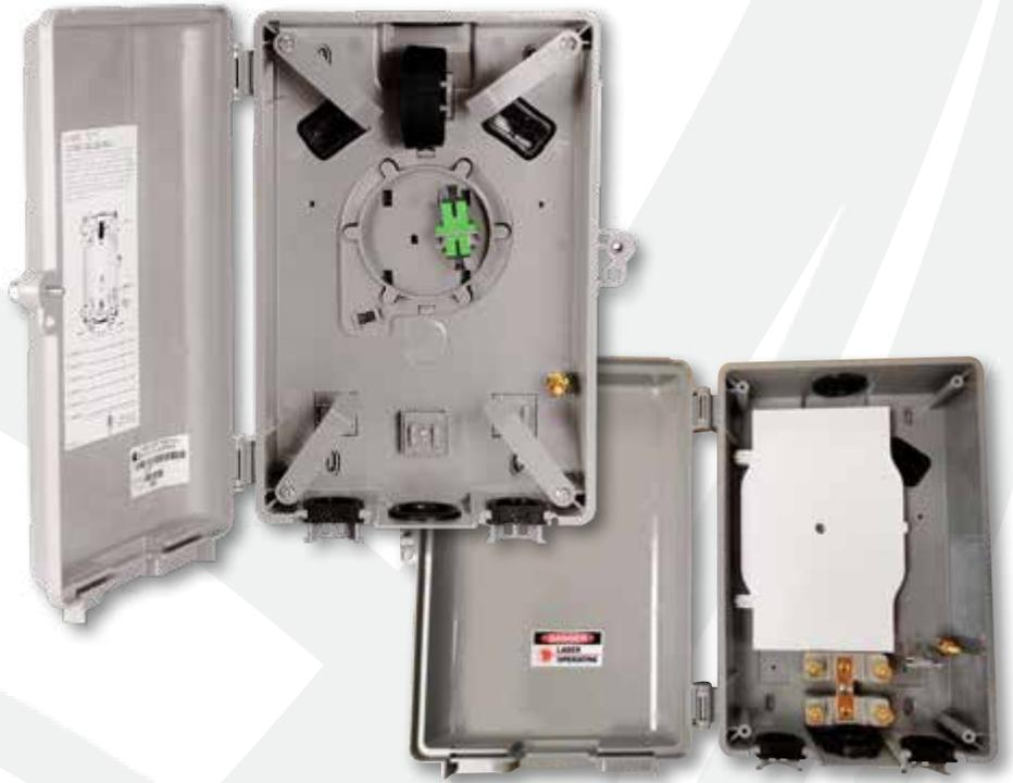
507F Fiber Interface Device/Slack Storage is a compact unit featuring connectivity between the OSP fiber drop and customer fiber drop, as well as slack storage for up to 50ft. of customer drop fiber. This unit accommodates multiple sizes of LB fittings and allows for termination through conduit at the top and bottom of the unit. The 507F is configurable for 1 to 12 fiber adapters.
