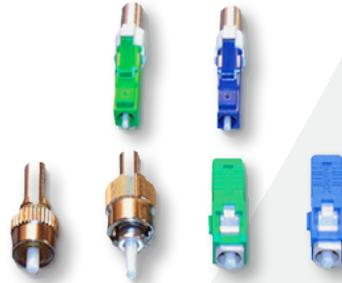
Optical terminators are used to terminate unused connector ports in fiber optic systems so that unwanted reflections are not introduced back into the system. Available in FC, LC, SC and ST.
