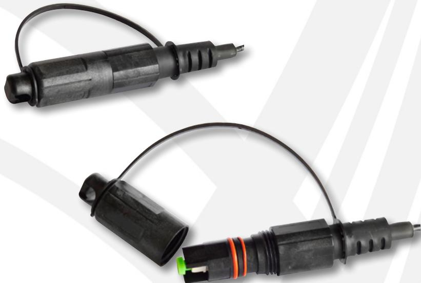
Tii's OptiFit Drop Cable Assemblies feature environmentally hardened, sealed and strain-relieved connectors that are factory-terminated on one or both ends of optical drop cables. These assemblies are custom made to required length to save service providers and installers considerable time and money when deploying FTTx networks and eliminate the need for fusion splicing for drop cable installation and subscriber connection.
