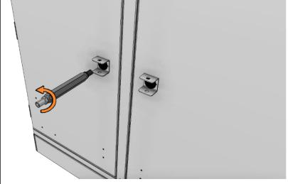
2.2 Open the doors until the locking pin snaps into their secure position
