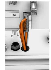
3.5 Insert distribution cable thru large cable port, tighten external nut and secure jacket with hose clamp.
