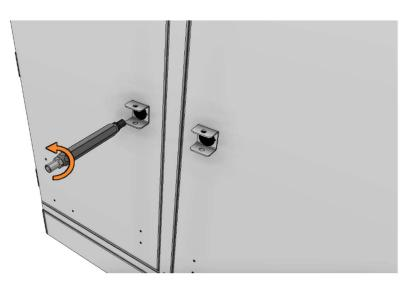
2.2 Open the doors until the locking pin snaps into their secure position
