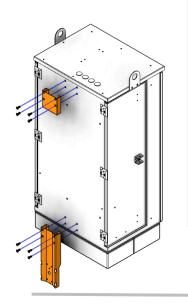
1.2 Mark on the pole the desired location of the cabinet top. Install the pole bracket 4.25 inches below that mark, with screws or metal straps.
