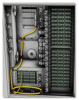
5.4 Connect splitter distribution legs to desired adapters on distribution field and route cable on provided management clips as needed.
