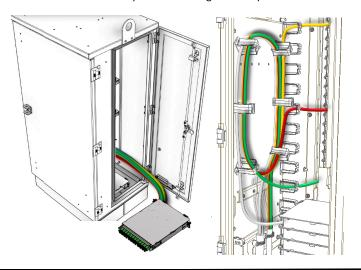
4.10 Reinstall cassettes by sliding into cabinet adapter first, rotating adapters towards front of cabinet, and securing into position by pressing the nylatch pin.
