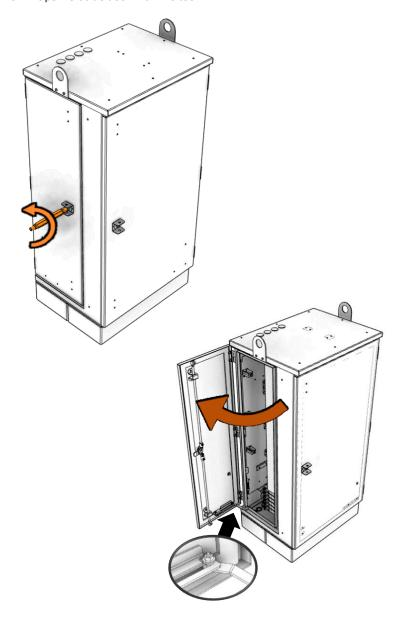
2.3 Secure with 3 screws from inside the cabinet as indicated above.
