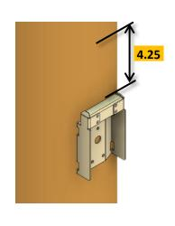
1.3 Hoist the cabinet from the two lifting ears and slide it over the pole bracket. Secure the bottom bracket to pole with steel straps or screws.
