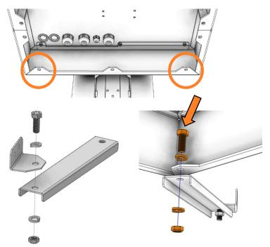
1.5 Attach L bracket of brace to the pole with provided  $1/4" \times 2"$  lag screws. Tighten the brace screws to secure position.
