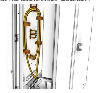
4.5 Insert distribution cable thru large cable port, tighten external nut and secure jacket with hose clamp.
