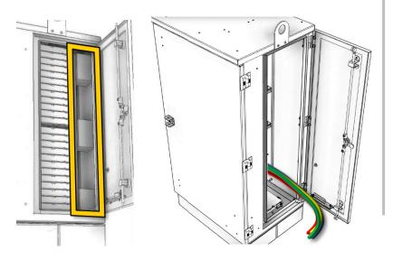
4.8 Remove the distribution cassette by releasing the mounting pin (located on the far side behind the cassette as shown), slide the cassette rearward, and remove the cassette through the side door opening.
