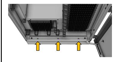
3.2 Bring grounding cable thru provided hole on bottom of cabinet, and securely fix to grounding bar.
