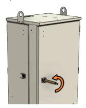
2. To install splitter onto mounting bracket, push top of mounting clip toward rear of cabinet. Catch
