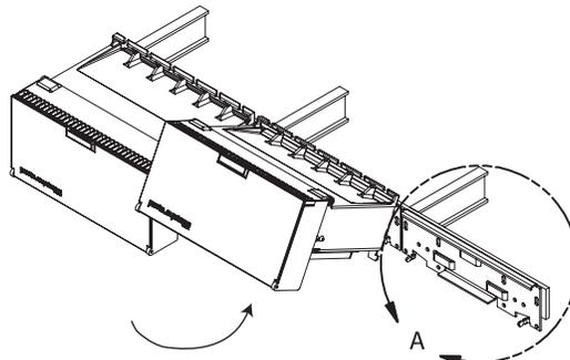
**Step 3:** Rotate downward to snap onto bottom side tabs.
