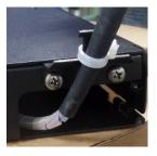
6. Secure feeder cable to cable entry clamp using supplied hose clamps or other suitable fastener like a zip-tie.
