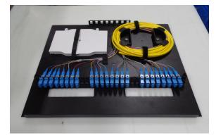
5. Remove master plate from front or rear to assist with fiber routing. Terminate or fusion splice feeder cable. Re install master plate with feeder cable. Store excess feeder in slack storage loop.
