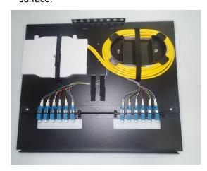
Remove master plate from front or rear to assist with fiber routing. Terminate or fusion splice feeder cable. Re install master plate with feeder cable. Store excess feeder in slack storage loop.
